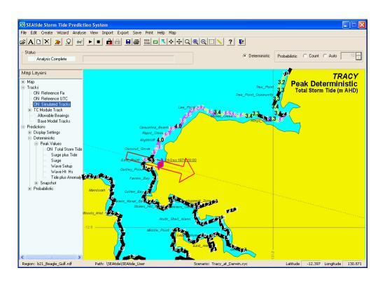
Deterministic parametric wind fields are combined with barotropic tide and surge modelling that is also then parameterised.
